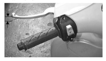
If the free plays do not fall within the limits, turn the right and left adjusting nuts for adjustment.
