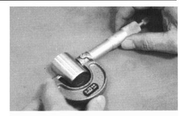
Check the caliper cylinder for scratch or wear and measure the cylinder bore.
