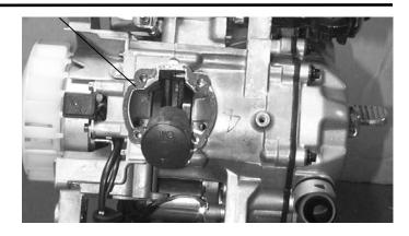
Make sure that the ring end gaps are aligned with the piston ring pins in the ring grooves.
