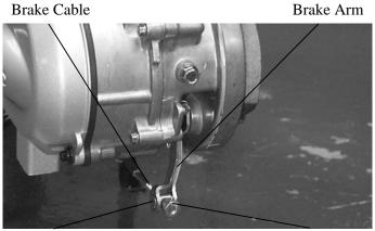
Brake Arm Pin Adjusting Nut
