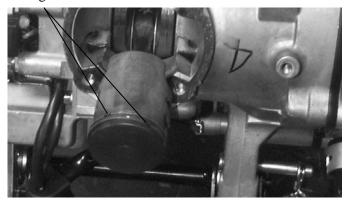
Install the cylinder head. **Torque**: 1.5□1.7kg-m
