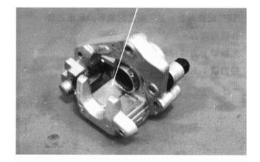
Remove the piston from the brake caliper. If necessary, use compressed air to squeeze out the piston through the brake fluid inlet opening and place a shop towel under the caliper to avoid contamination caused by the removed piston.
