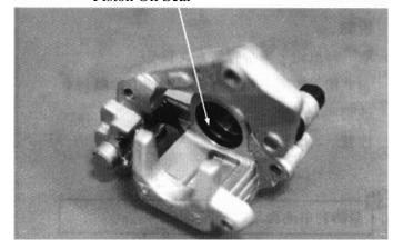
Check the piston for scratch or wear.
