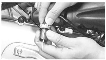
Remove the throttle valve spring, carburetor cap and rubber seal.
