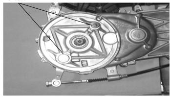
Apply engine oil to the felt seal and install it to the brake cam.
