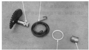
Plastic Bushing Spindle Bushing
