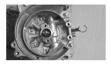
Attach the crankcase puller on the right crankcase and remove the right crankcase from the left crankcase.
