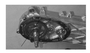
Install the countershaft and gear into the left crankcase.
