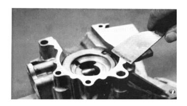
Drive a new crankshaft bearing into the right crankcase.
