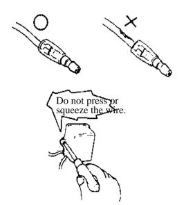
■ After routing, check that the wire harnesses are not twisted or kinked.
