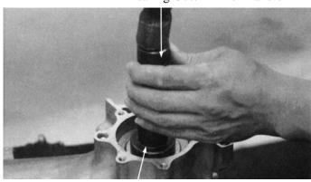
Bearing Outer Driver, 42x47mm Pilot, 20mm
