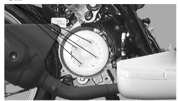
When the engine is running at the specified rpm, the ignition timing is correct if the "F" mark on the flywheel aligns with the index mark on the crankcase within  $\pm 1.5^{\circ}$ .
