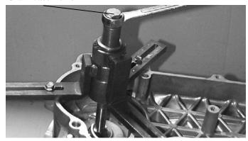
Remove the remaining bearing on the crankshaft side using the universal bearing puller.
