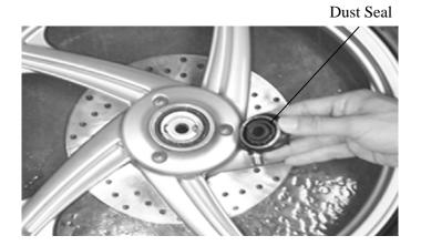
Remove the wheel bearings and distance collar.
