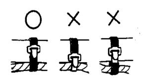
■ After clamping, check each wire to make sure it is secure.
