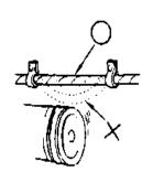
■ When fixing the wire harnesses, do not make it contact the parts which will generate high heat.
