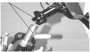
Lubricate the throttle pipe front end with grease.
