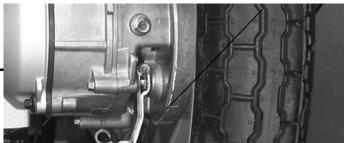
check if the front brake fluid level is within the specified limits through the front brake master cylinder check hole.
