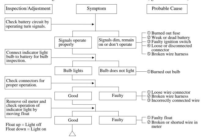
2. Motor oil is sufficient but the indicator light remains on (Ignition switch ON)
