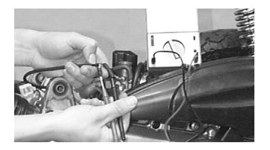
After the engine stops for 30 minutes, connect a hose to the fuel enriching circuit and blow the hose with mouth.
