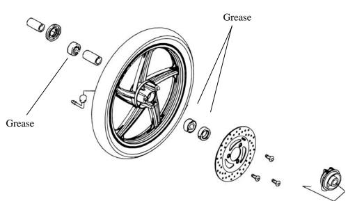
Pack all bearing cavities with grease. Drive in the left bearing. Install the distance collar. Drive in the right bearing.
