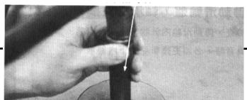
Set the driven pulley, driven face spring and clutch assembly onto the clutch spring compressor. Compress the tool and install the
