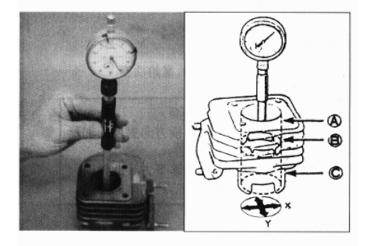
Inspect the top of the cylinder for warpage. **Service Limit**:
