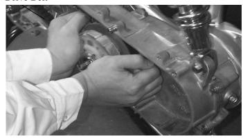
Set the drive belt on the drive pulley. Install the drive pulley face, starting ratchet and 12mm washer, then tighten the drive face nut.
