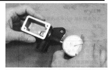
Measure the brake master cylinder piston O.D.
