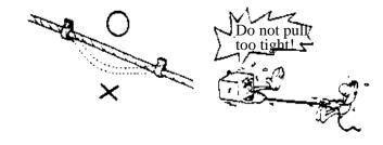
■ Protect wires and harnesses with electrical tape or tube if they contact a sharp edge or corner.
