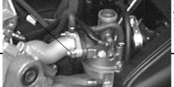
Connect the auto bystarter yellow wire to the battery positive (+) terminal and green/ black wire to the battery negative (-) terminal and wait 5 minutes.
