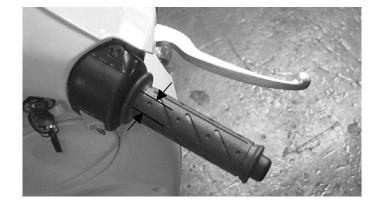
If the throttle grip free play does not fall within the specified range, adjust by loosening the lock nut and turning the adjusting nut.
