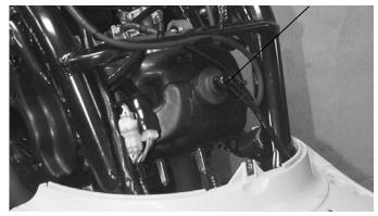
Remove the spark plug cap. Remove the three bolts attaching the fan cover to remove the fan cover.
