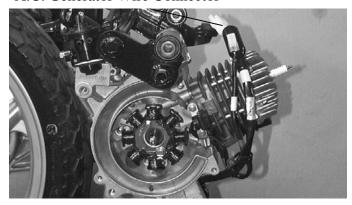
Remove the two pulser coil bolts and pulser
