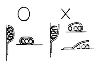
■ Do not squeeze wires against the weld or its clamp.
