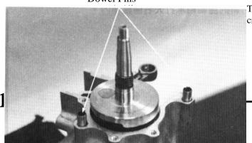
The distance between the left crankcase oil seal and crankcase surface is about 1.0mm.
