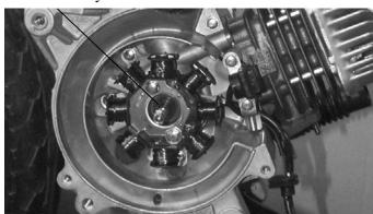
Install the flywheel onto the crankshaft with the flywheel groove aligned with the crankshaft woodruff key.
